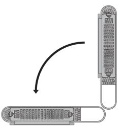
**5** The receiver is ready. Make sure that the front side (with the LED indicators) of the receiver is facing you.
